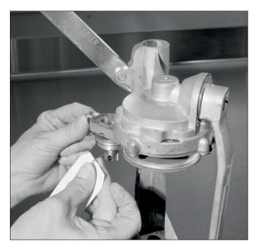
Make sure the "2" appears in the indicating window. Insert the **THIN/SMALL** gauge wire between the chuck and the groove in the second seaming roller.
