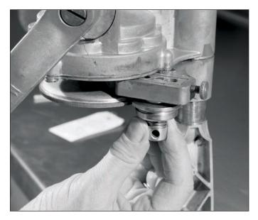
Finger tighten the first seaming roller screw. This removes slack yet allows the roller assembly to slide with rotation of the thumbscrew.
