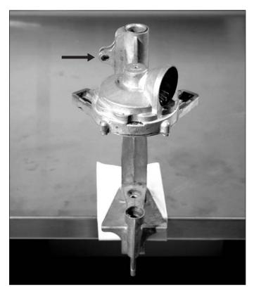
The head drops onto the frame. Notice that there is a slot both in the head and in the post of the frame (arrow).
