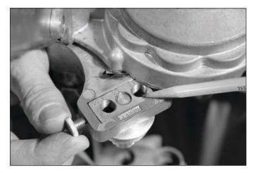
Rotate the crank until a "2" appears in the indicating window. Install the second seaming roller on the left side in the same manner as the first (see pages 17–19). Note the orientation of the 3-hole nut (pencil points to the #1 hole).
