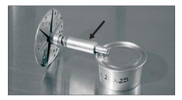
Select the required spacers and extension for your can size (see page 14). Place the spacers, then the spring onto the shaft of the turntable. For the 307 x 200.25,  $V_2$ -pound flat salmon can, the turntable extension is required (arrow).
