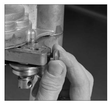
Thread in the thumbscrew loosely. Rotate the crank until the "1" appears in the indicating window.
