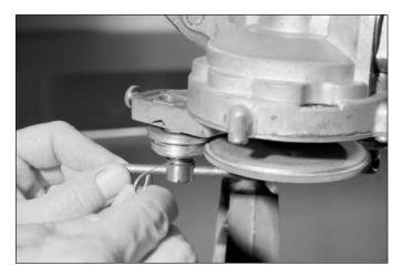
Lock the seaming roller screw in place by tightening with the 3-inch pin. Draw (lightly pull) again on the gauge wire—it must not move easily. If it moves, loosen the seaming roller screw slightly and tighten the thumbscrew slightly. Repeat until the gauge wire cannot be moved easily.
