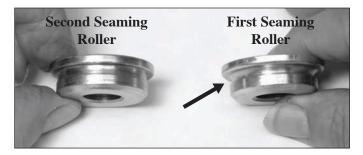
There are two seaming rollers. The "first" seaming roller is on the right side of the sealer and is for curling the lid and can body edges together. This roller has a deeper, more rounded profile.
