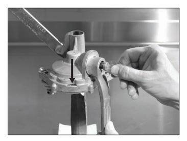
Finger tighten the screw. Turn the crank handle until the "0" appears in the center of the indicating window (arrow).
