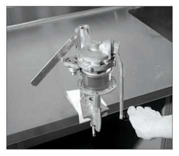
Steadily rotate the crank clockwise through the entire cycle, starting and ending at "0" in the indicating window. The indicating window will display "0," "1," "C," "2"—then back to "0" in a complete can seaming operation.
