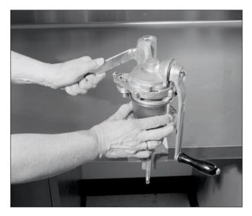
With the can and lid in the center of the turntable, slowly lower the lever, moving the can as necessary to keep it centered. Press the lever down to the locked position. This WILL, AND SHOULD require some force as you compress the turntable spring.
