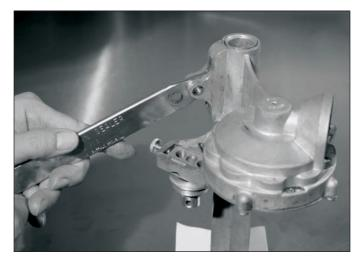
Place the head on the frame post. Align slot in the head with the slot in the frame. Insert the lever into the slot (writing should face forward). Line up the hole in the lever with the two holes in the head.
