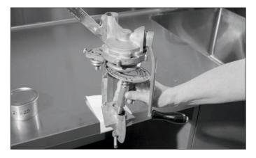
Situate the turntable by lifting the can sealer lever to the up position. Insert the turntable into the frame.
