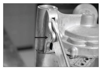
The lever pivot should be flush with the backside of the head (arrow).
