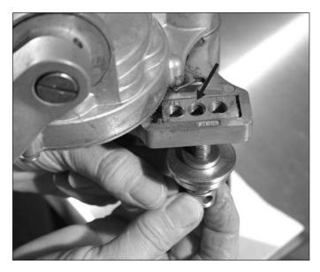
Loosely thread the first seaming roller assembly into the 3-hole nut from the bottom.
