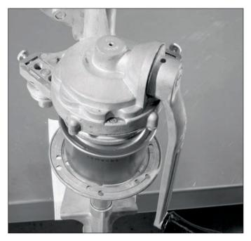
Begin with the "0" in the indicating window and the crank hanging straight down. Raise the lever to the full up locked position. Center a can on the turntable. Then center a lid (gasket down) on top of the can.
