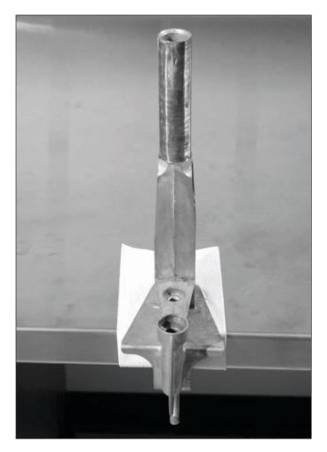
Start by clamping the frame securely to a table. Use the 3-inch pin to tighten the clamp screw. Use a cloth or a piece of cardboard to protect the surface of your table.
