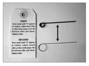
Accurately setting and securing both seam rollers is essential. The first and second gauge wires are used to set the distance between the rollers and the chucks. These settings control the shape and tightness of your can seams—and therefore the quality of the hermetic seal. Since food must never be stored in cans that have improperly formed seams, an improperly adjusted can sealer has no role in food preservation.
