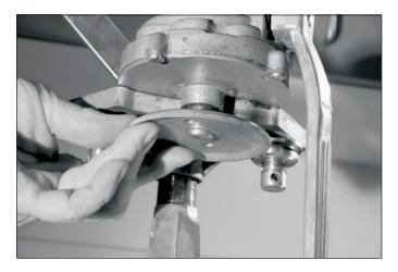
Rotate the crank until the "0" appears in the indicating window. Select the appropriate chuck for the can size you will be using (see page 14). With the concave face of the chuck facing down, insert the chuck screw through the center of the chuck. Thread the screw into the head by hand. Do not use a screwdriver.
