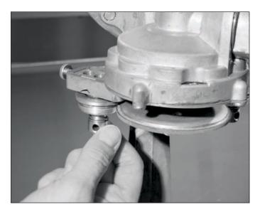
Move the seaming roller to the outside by sliding the 3-hole nut until it stops hard against the frame.
